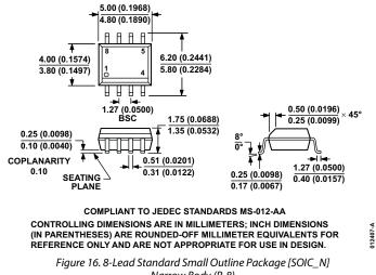
Narrow Body (R-8) Dimensions shown in millimeters and (inches)
