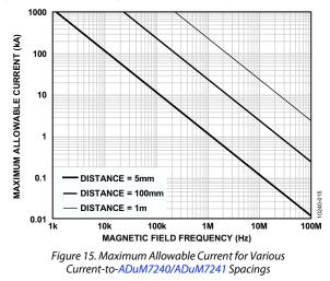
Note that with extreme combinations of strong magnetic field and high frequency current, loops formed by printed circuit board traces can induce error voltages large enough to trigger the thresholds of receiver circuitry. Care should be taken in the layout of such traces to avoid this possibility.
