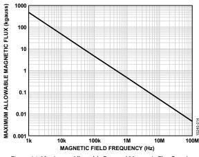
Figure 14. Maximum Allowable External Magnetic Flux Density
