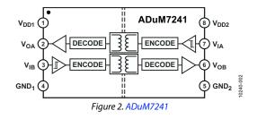
ADuM7240/ADuM7241 provide low pulse width distortion (<5 ns for C grade). In addition, every model has an input glitch filter to protect against extraneous noise disturbances.
