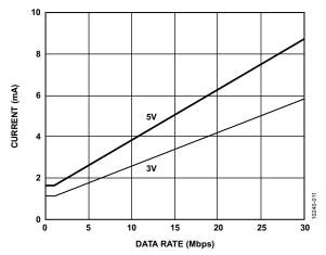
Figure 11. Typical ADuM7241 V<sub>DD1</sub> Supply Current vs. Data Rate for 5 V and 3 V Operation
