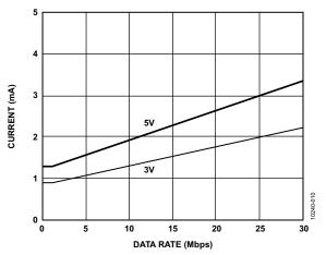
Figure 10. Typical ADuM7240 V<sub>DD2</sub> Supply Current vs. Data Rate for 5 V and 3 V Operation
